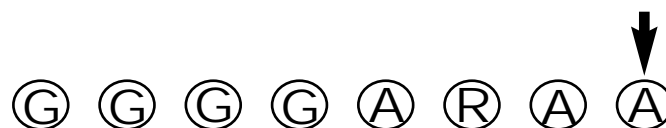
Figure 17 - Indicates entry into the Advanced System Voltage Adjustment mode.
