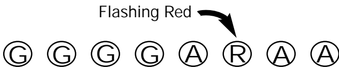
Figure 32 - Indicates activation of diagnostic mode. Diagnostic codes are shown in Figure 33 at right.
